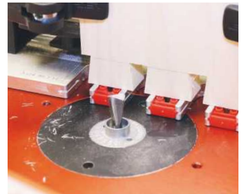
▲ The pegs prevent the guide bush from making a cut
